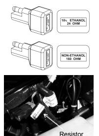
**NOTICE:** Engine damage may occur if ethanol fuel is used while the non-ethanol fuel resistor is installed. The check engine light may also display in this condition as this could cause detonation.
